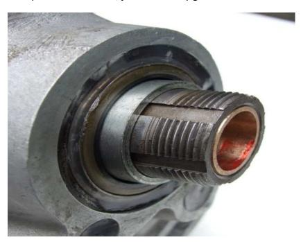
If you have an old oil seal ring (a new one comes with the POC kit) also put this on the shaft and it will allow you to put the large sprocket nut on, giving you something to grab hold of when testing the gearbox on the bench, and will also stop the loose new ring from falling out. Alternatively loosely fit the chain sprocket.
