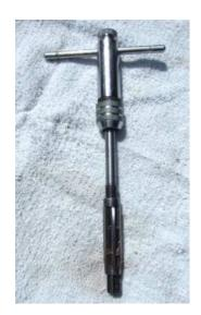
The bush bore now needs to be reamed to match the diameter of the Layshaft – your Layshaft may have suffered wear in the past and been ground undersize – in fact the two ends may even differ in size, so make sure that you are matching to the correct outer end of the Layshaft when reaming. Mine were 2 thou different in diameter.
