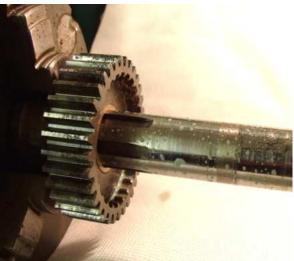
Unless you can find out what Burman originally recommended and also have the means to accurately machine and measure to those tolerances, then 'free-running, with barely discernable play' could be the choice — Oilite bearings of the diameter found in this gearbox fall into the range of 2-3 thou" clearance. Remind yourself that this is a 60 year old gearbox and no Rolex wrist-watch!
