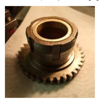
As my main shaft had 3 thou wear and the best I could achieve was to ream the bushes to match the original shaft diameter, plus a thou to let me get it onto the shaft, allowing the unworn part of the shaft to be a sliding fit through the bush.
