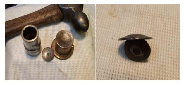
Make sure the seatings for these are oil-free and apply a thin bead of sealant. Use a tubular drift such as a socket just and lightly tap the dics down, dome upwards, until they just contact the bushes.
