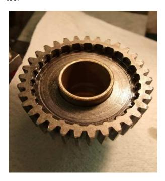
The only new bushes available are oversize both in outside diameter and bore (28.6mm x22.1mm), whereas the ones that came out were smaller in outside diameter and larger in bore (27.75mm x 22.85mm (worn!)).
