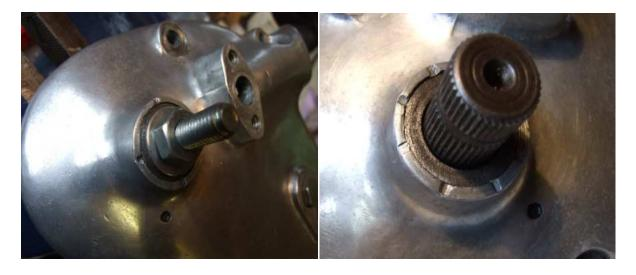
**1.2 Fitting the clutch lever** is the reverse of removal – it will need further adjusting once the clutch cable has been re-fitted. Don't fit the small outer adjuster casting at this stage.
