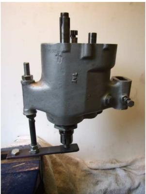
If you have used the vertical jig (assembly is very, very easy with it) then raise/adjust the main casing upwards and support the end of the mainshaft on the lower part of the jig, with all of the weight of the casing being taken on the vertical stud, and the mainshaft projecting around 3/4" from the mainshaft sleeve.
