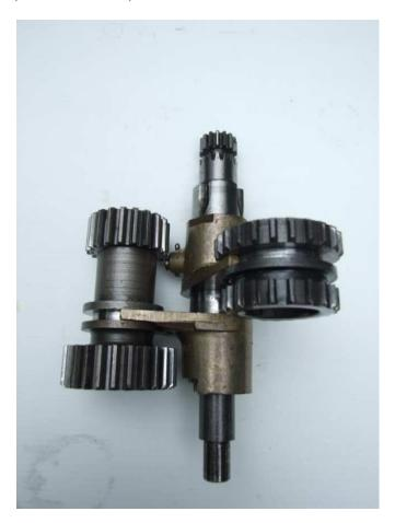
Set the selector shaft into its bush at the bottom of the gearbox, and then spread the gearsets apart, supported by the selector forks. Look down through the Layshaft gears and line them up with the Oilite bush that you'll be able to see in the bottom, and feed (and wriggle) the Layshaft fully into place. The Layshaft has splined ends and it's the longer spline that goes in first.
