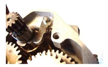
Put a thin smear of Hylomar type sealant on the main case, apply the gasket (my home-made gasket was 0.25mm thick), and use Hylomar on the inside face of the mid-section casing.
