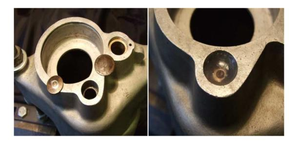
Then, using a large diameter plain drift, tap the centre of the dome of the disc to spread it out – there is no need to flatten or batter the disc, just a couple of centrally placed light taps. Once in place, fill the remaining bore with sealant and smooth the outer face with a wet finger. Wipe any excess sealant from within the bearings.
