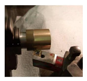
If you do it yourself then turn the bush outer surface to the diameter of your gear bore plus around 3 thousanths of an inch, so that the bush will be a tight press fit in the main gear. You'll need to make up a simple mandrel for the bearing to sit on for machining—I used a piece of aluminium bar turned so that the bush just tapped over it, as in the photo. If you try to use the expanding chuck jaws the bush will distort, becoming triangular.
