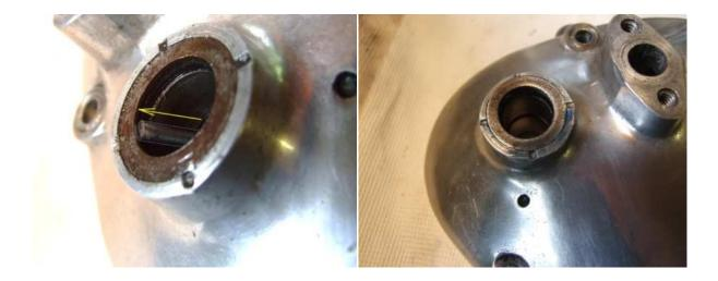
Place the larger O ring in place and run a thin bead of Loctite around the washer seating and put the washer in place. It will be held up too high by the O ring. Use a piece of studding and pull the washer fully onto its seat, compressing the O ring. Leave the studding in place and peen over the casting in 4 new places to retain the washer, which, along with the cured Loctite will hold the O ring securely. Smear a small amount of grease onto both O rings and bushes.
