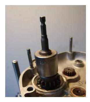
**4.8** Apply another good dose of oil to the exposed bushes & bearings and then fit the selector quadrant assembly.
