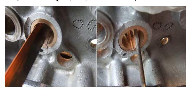
Cut a 1mm deep line into the bush with the saw, remove the blade and use a coarse rat-tail file to open up a neat trough. Don't be tempted to run the reamer back through once the groove has been cut — it will chatter as a result of the groove. Thoroughly clean the casing of all swarf prior to fitting the ball race.
