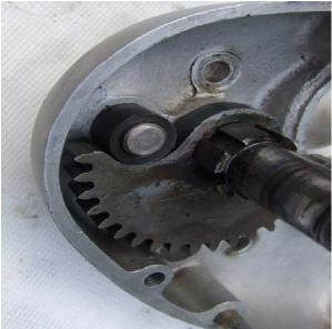
(Before fitting the kickstart spring to the outer casing test clearances by putting the outer case and mid section of the gearbox together to make sure that the cases are not being held apart at all. I found with this gearbox that the kickstart shaft could be felt to bind when the cases were pulled up together without a gasket, so clearly a gasket, rather than sealant, was the best option. I made a gasket from 0.5mm gasket paper, but they are available from POC.
