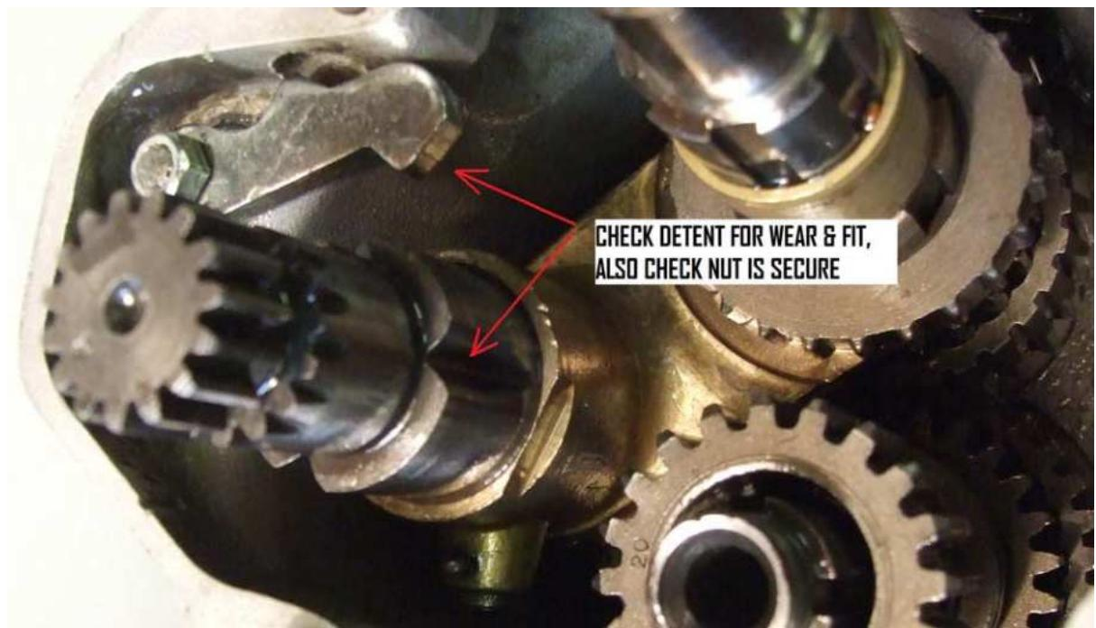
Check detent spring for length & distortion – these are available from POC.
