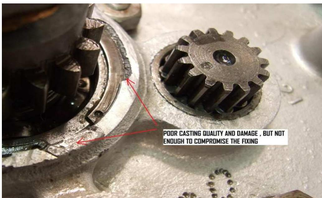
The next one needed a lot of thought! This was the back of the middle casing, outer mainshaft bearing housing . It's not there! Possible causes may have been the bearing being pressed into place without supporting the back of the casting, or levering the clutch hub off of its splines. It needed professional expertise.
