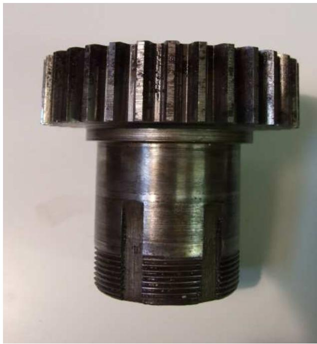
The gear teeth may have eroded areas, chips, cracks etc and every one needs close inspection. The most likely symptom will be noise, but a broken off tooth might have done a lot of damage.
