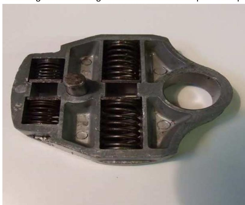
The selector pawl assembly is riveted and the 3 rivets needs to be secure – if you need to tighten yours make sure that the shaft is in place to keep everything centred on the single rivet, otherwise you risk making it very secure , but in the wrong position.
