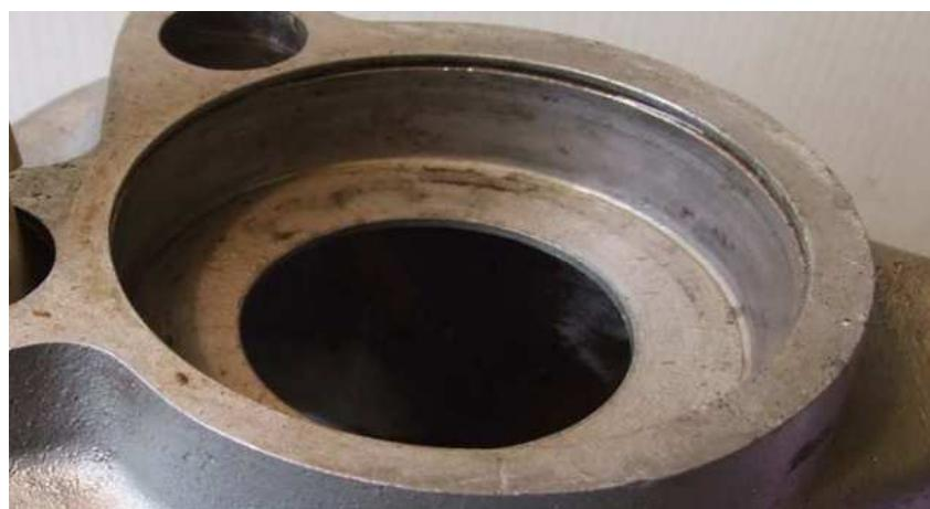
Circlips available from bearing suppliers – take the casing and old clip along if you have a local supplier.
