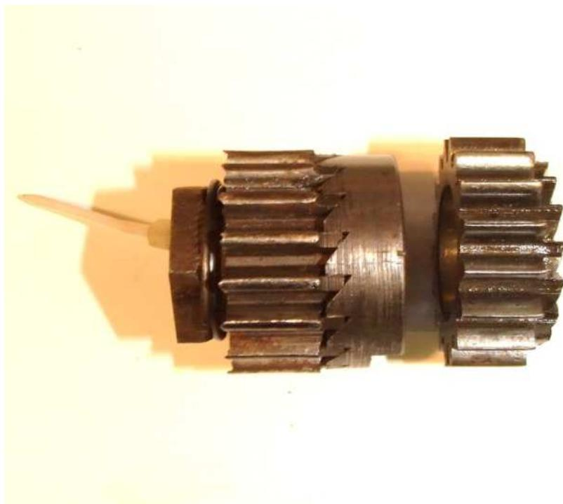
Look at the end of the layshaft when in situ and push it sideways with a screwdriver – you'll hear the oil 'click' as it gets pushed out of a worn bearing. New bushes are readily available
