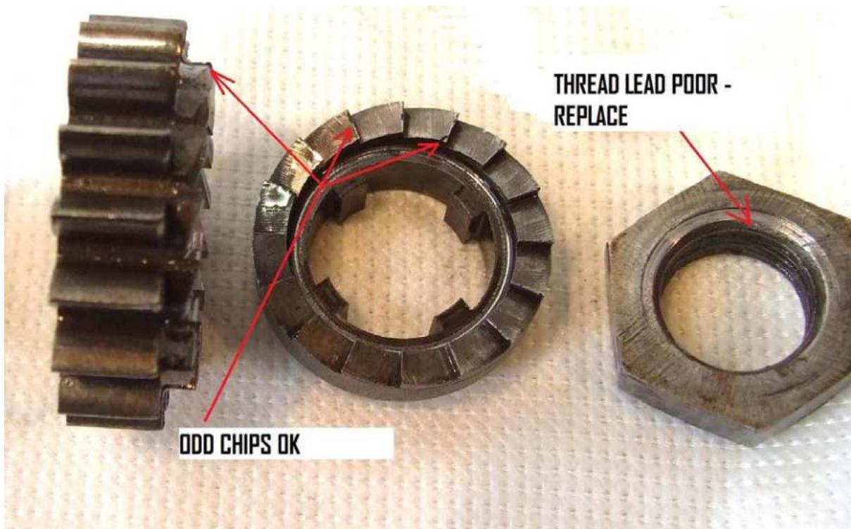
If in poor condition the above assembly is available new from POC, and the spring dimensions when new are 19mm L x 27.5mm O/D.
