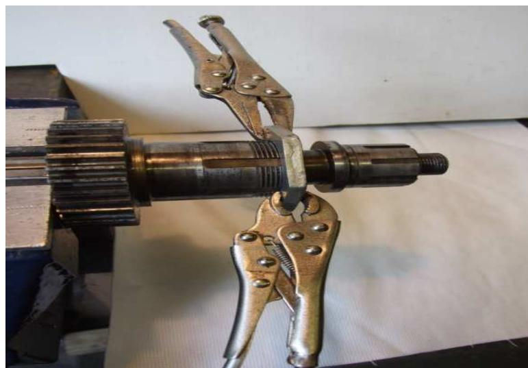
Rock the drive gear on its bearing and the movement will be similar to the rock that is found at the clutch sprocket teeth. I set up a dial gauge, and, on a ‘moderately’ worn bearing/shaft, there was 20 thou+ movement at the same diameter as the clutch –
