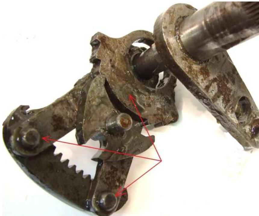
The selectors within the gearbox can become bent or worn and there's not much that can be done by way of repair, so better replacements will need to be found. This looks like a replacement as it's in good condition. There is no great need to dismantle this assembly if the selectors are serviceable.
