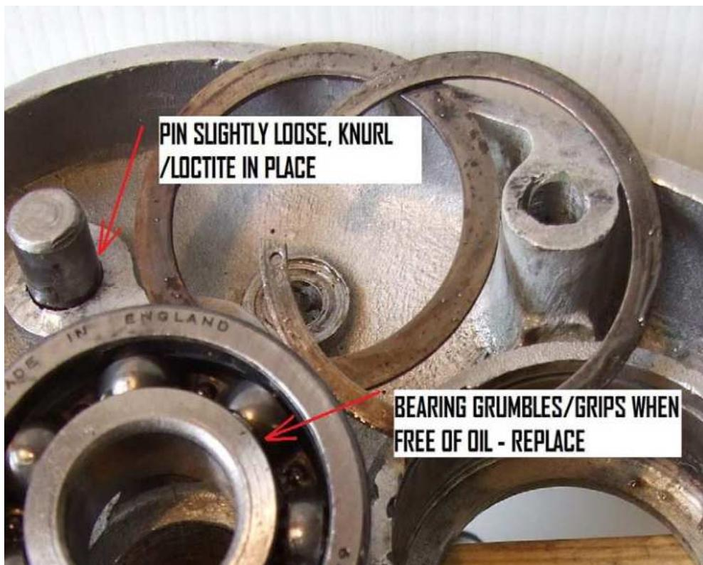
As with any accessible bearings, if in doubt, replace. This outer main bearing, relatively new, initially felt OK, but a wash out with a squirt of carb cleaner revealed that it didn't spin smoothly, and a judder could be felt as it slowed, so maybe some pitting. Available from POC and is a standard metric bearing, SKF 6304, held by all bearing suppliers and widely used on agricultural equipment, as are new circlips.
