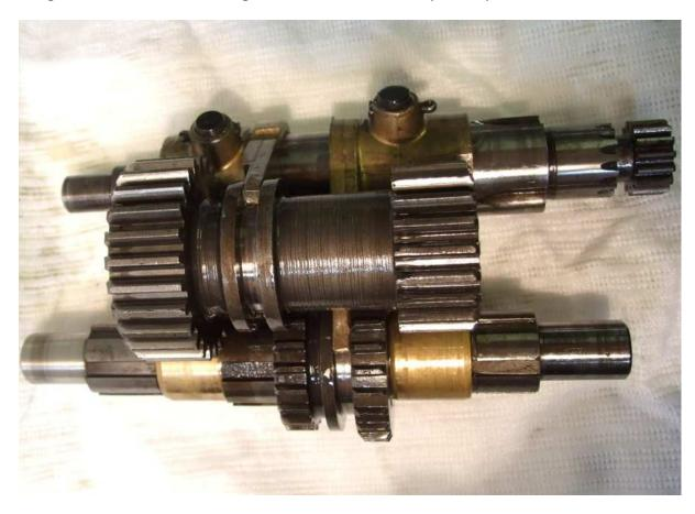
Still inside the gearbox is the large mainshaft drive gear to the left in picture and 2 loose layshaft gears to the right (a smaller one is out of sight here). Remove the layshaft pair first. The mainshaft gear has a sleeve which passes through the centre of the large mainshaft bearing located in the casing. Draw the gear upwards and recover the loose outside metal sleeve, which will either fall out or sit in the centre of the outer oil seal.
