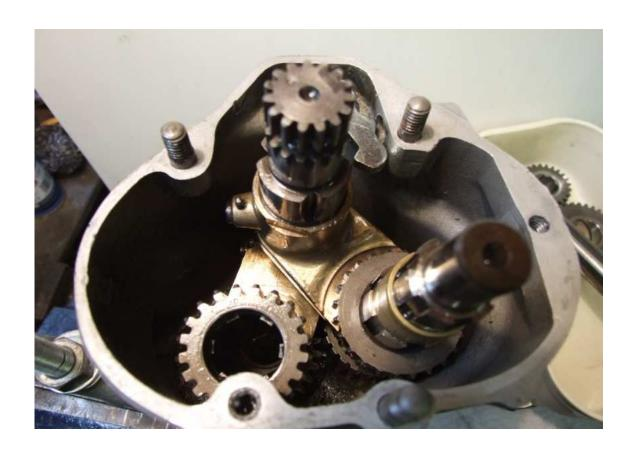
The gear cluster – this is how it goes back in on reassembly. It'simpler to do than it looks.
