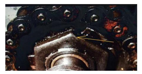
However if the nut looks decidedly second-hand (maybe even before you start!) then budget for a new one, and certainly a new lock washer from POC spares. Heating for a few minutes with a hot air stripper may help, especially if you suspect Loctite. Pull the sprocket off.
