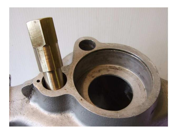
Oilite is quite weak and porous, and damages/distorts easily – it's the metal equivalent of Weetabix. You won't be able to re-use this removed bearing, so be certain that it does need replacing before knocking it out. Keep the old bush as a reference as the POC ones need reducing in length. Any replaced Oilites will need reaming to size— it's not a difficult nor expensive job and shouldn't put you off replacing them- all shown in the **Rebuild** section.
