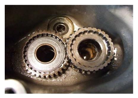
The same 2 gears removed below, mainshaft gear turned over to show splined drive sprocket sleeve plus 2 layshaft gears.
