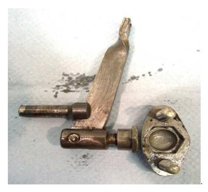
Keep all of the outer cover components together for cleaning and inspection.
