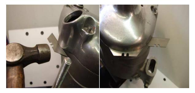
Work steadily around the cases, rotating the blades around the studs, until the whole outer cover has moved away from the inner. Find a couple of flat pieces of scrap to gently lever the cover upwards – I used 2 brass Rally Plates here, and increase the gap to a few mm. until you are sure that the sealant has been cut through. Remove all blades / plates
