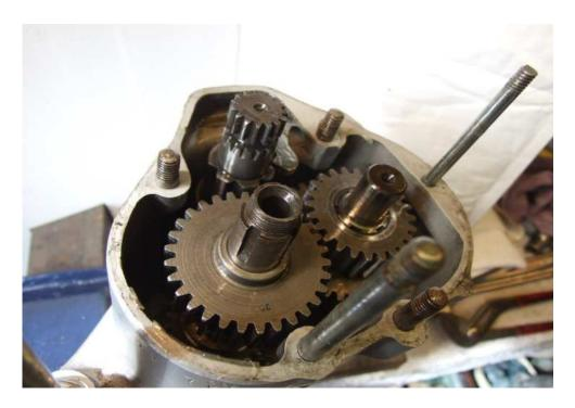
If you rotate the selector shaft a little either way you'll see the gear dogs lift & fall to engage/disengage gear sets. To the right of the selector shaft is the (silver) detent peg, operated by the spring that you earlier removed, which matches the various gear selector positions. It is held in place by a small nut and this should not be disturbed unless replacement is necessary.
