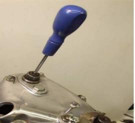
Find a screwdriver – (a Philips will fit well), and push it into the threaded hole that is in the centre of the gear shift shaft. This will be used to hold the shift assembly in place whilst you remove the cover – the whole splined gear shift shaft passes through the cover, and is left in place as the cover comes off, whereas the complete kick start assembly, held by the Mole Grips, comes off with the cover.
