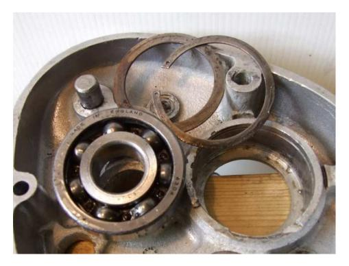
If the kickstart stop pin (shown 11 o'clock above bearing race here) is bent / damaged /loose this can also be tapped out from behind.
