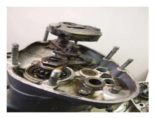
And, inside the front cover, the clutch lever assembly and, still coiled, the kickstart spring
