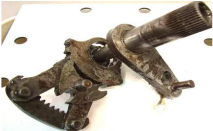
It leaves exposed the toothed selector shaft , beneath which can be seen the loose rollers that act as a bearing, sitting captive in a groove in the selector shaft.
