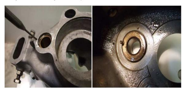
Working from outside, using a drift (ideally stepped, dimensions as shown) push/tap the Oilite bush into the hot casing until it drops out. The same drift is used in replacement.
