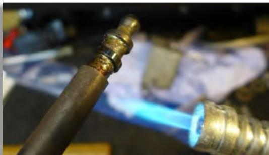
Figure 21: Soft soldering with a blow torch.
