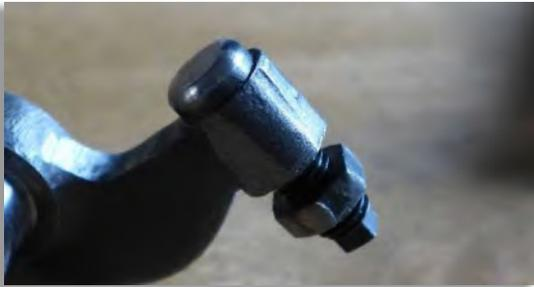
Figure 16: The inlet tappet at its rocker arm. As for the exhaust tappet its face radius matches with the arm length. However, the outer part has been once unnecessarily ground off.
