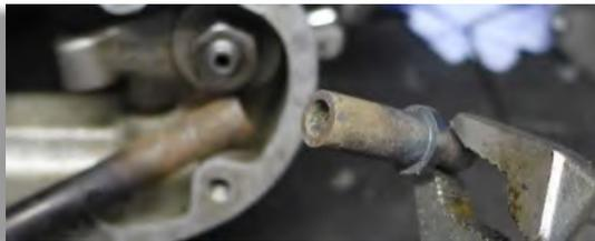
Figure 19: The ball section separated from the pushrod.
