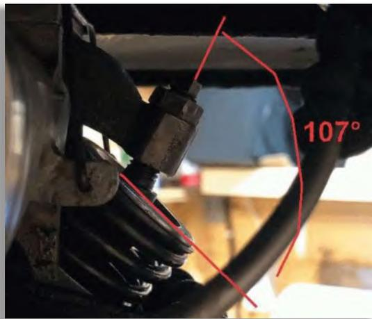
Figure 4: Rocker-to-valve angle for the closed valve.
