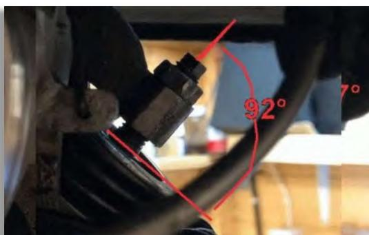
Figure 5: Rocker-to-valve angle for the open valve
