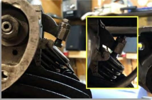
Figure 9: The outer rocker arm position after lifting the rocker box by 2mm. Inset: The situation before.
