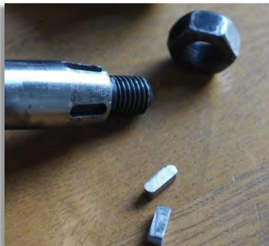
Figure 14: The tapered rocker shaft end with the two key ways and the new keys.
