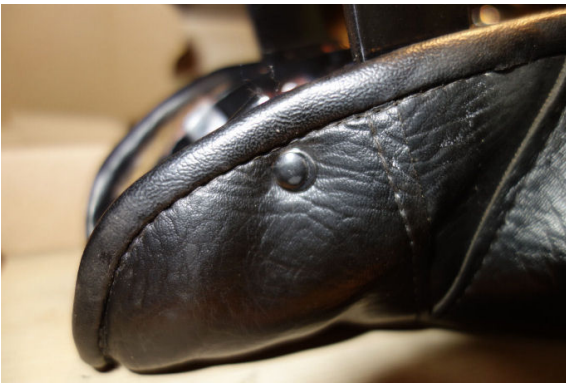
Figure 5 – Washers below the rivet heads.
