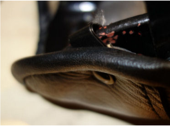
Figure 4 – The saddle clamps bent around the saddle frame.
