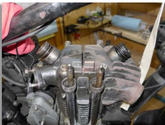
Figure 8: The cylinder head without the rocker box.
