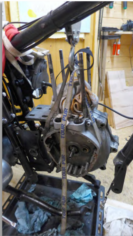
Figure 29: The crankcase in the hoist before dismantling the front carrier plates. The motorcycle was lifted down onto a trolley.
