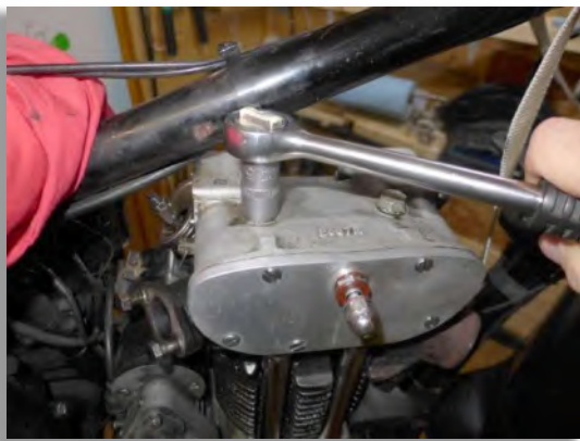
Figure 7: Loosen the bolts of the rocker box.
