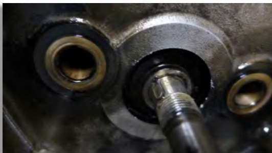
Figure 15: A perpendicular key on the crankshaft defines the unambiguous position of the timing gear.
