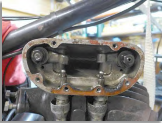
Figure 6: The rocker box on top of the cylinder head. Note the cups for the pushrods at the rocker arm ends. The rocker box cannot be shifted aside until the pushrods are lowered.
