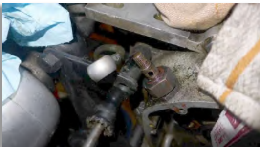
Figure 23: Disconnected vent pipe at the timing cover.
