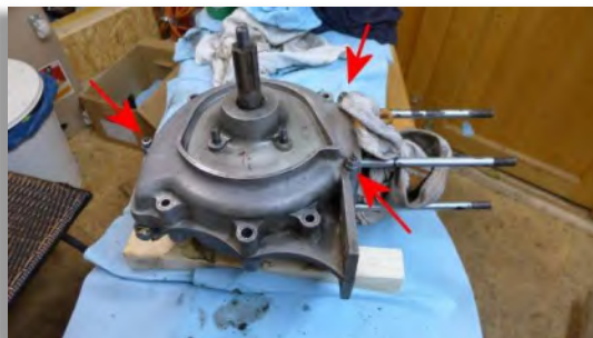
Figure 32: The crankcase on the bench without the rear carrier plates. The arrows indicate the three bolts which hold the two halves together.
