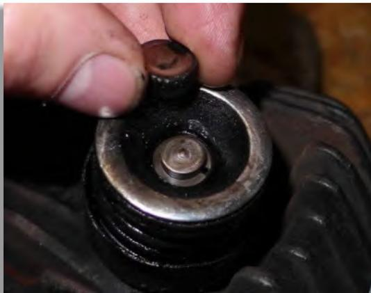
Figure 17: A hardened valve cap on the valve tip. New caps should be made out of silver steel with an inner diameter to a good fit to the valve tip. The top material thickness is 0.06". Then harden and temper.
