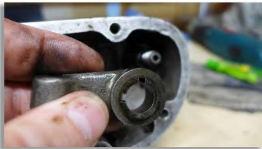
*Figure 13: The loose inner rocker arm with its two grooves for the keys.*
