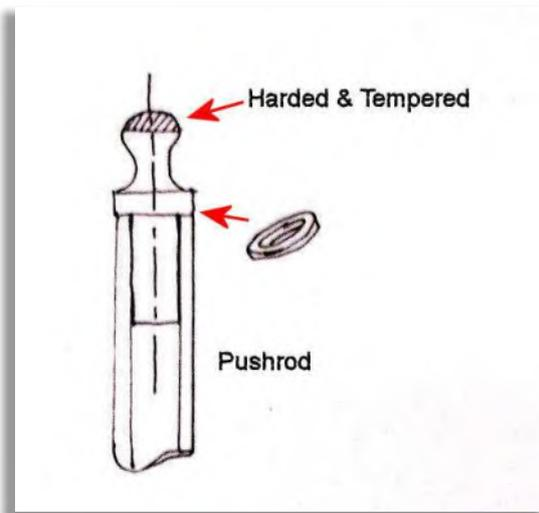
Figure 7: Drawing of the pushrod and the packing ring. The ball ended insert is soft soldered into position. A packing ring out of silver steel can be inserted to adjust the pus rod length. The ring and the ball section (indicated) should be hardened and tempered. Courtesy Chris Odling.
