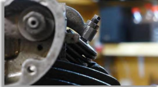
*Figure 23: The final rocker arm geometry for the closed valve.*
