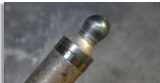
Figure 22: The finished pushrod with the distance ring.
