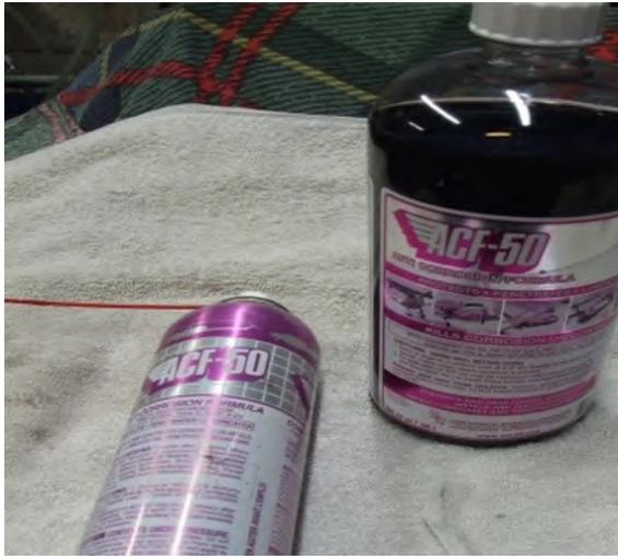
Great on bare steel – lathes, hand planes etc., but keep it away from brake surfaces as it is also a lubricant. Over time it will gather dust, but still stops any corrosion – just an annual wipe off and a fresh coat keeps things looking good. Alternatively dry the parts thoroughly & prime and top-coat them as soon as possible after the electrolysis treatment.
