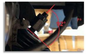
Figure 5: Rocker-to-valve angle for the open valve
