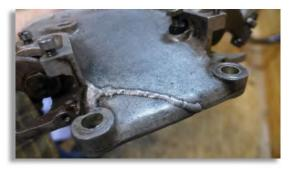
*Figure 8: The welded upper part of the rocker box.*
