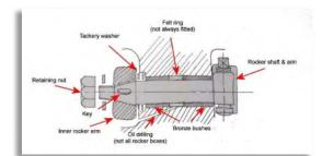
Figure 10: Drawing of the rocker assembly. Courtesy Chris Odling.
