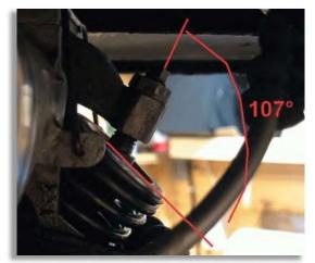
Figure 4: Rocker-to-valve angle for the closed valve.
