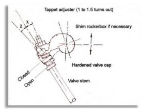
Figure 3: Sketch of the rocker geometry when it works nominally. Courtesy Chris Odling.
