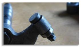
Figure 15: The exhaust tappet at its rocker arm. Its face seems to be flat at first sight but has a radius matching with the arm length.
