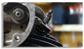
*Figure 23: The final rocker arm geometry for the closed valve.*
