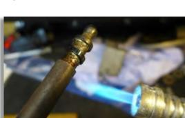
Figure 21: Soft soldering with a blow torch.
