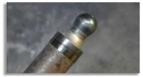
*Figure 22: The finished pushrod with the distance ring.*
