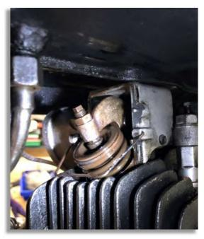
Figure 2: The exhaust valve spring covered by the same brown oil.
