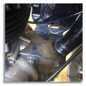
Figure 1: Brown oil on the lower motor mount cover indicated a problem with the valve guide.
