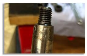
Figure 12: Worn keys in the shaft key ways.
