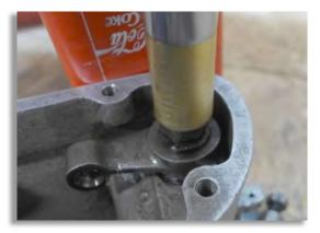
Figure 11: Applying a brass punch to loosen the inner rocker arm from the tapered shaft.
