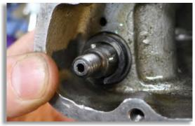
Figure 18: The new keys in the rocker shaft.
