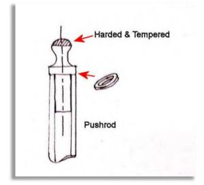
Figure 7: Drawing of the pushrod and the packing ring. The ball ended insert is soft soldered into position. A packing ring out of silver steel can be inserted to adjust the pus rod length. The ring and the ball section (indicated) should be hardened and tempered. Courtesy Chris Odling.
