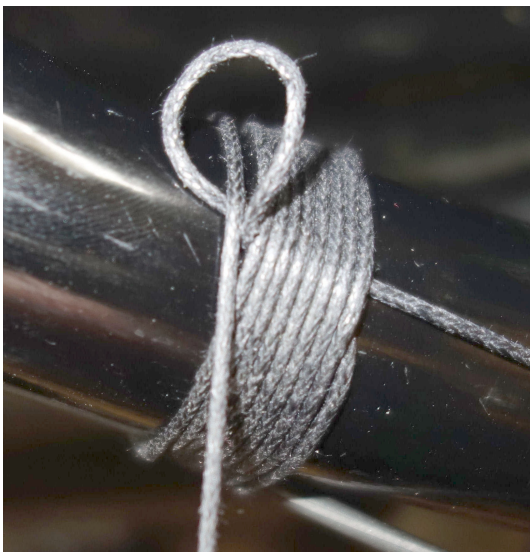
Figure 6: The string end is pulled through the open loop and then closed by pulling the other string end.
