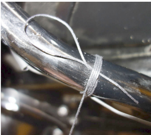
Figure 5: Winding the longer cord end around the frame and the cable.
