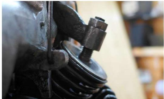
At home I found that the surface hardening of the exhaust side follower was breached and worn. Through emails and phone calls with Chris Odling, I learned that an oil feed to the exhaust valve guide is not necessary. Such engines run "oily" and one can feel it on the oily soot with fingers. On the later Sunbeam motorcycles like mine from 1937, it was common that only the inlet valve was lubricated. And bronze, often used for modern machines, is not a suitable material because
