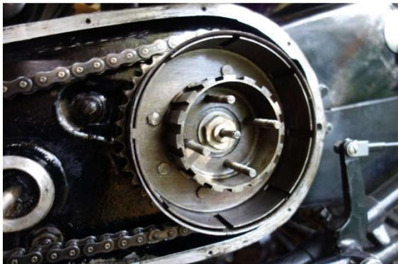
All clutch plates must first be removed for inspection. The basket/sprocket assembly is then disconnected. To do this, a lock washer must be removed and a large 26mm nut loosened with a socket wrench. **Caution:** If the clutch assembly is then pulled out, 24 bearing rollers will fall out. In order not to lose the rollers, one should catch them with a tray underneath (I took a baking tray).
