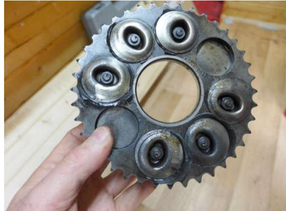
The rollers can be reassembled later with grease to hold them. If one turns the basket/sprocket unit upside down, the rubbers can be found in corresponding holders under metal plates with elliptical recesses for the nuts. The nuts are normally held by grit holes that widen the bolt head. This is important to prevent the nuts from coming off during driving, which would have fatal consequences. When reassembling the bolt, either one puts a new punch with a center punch or one uses Loctide.
