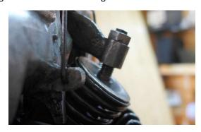
At home I found that the surface hardening of the exhaust side follower was breached and worn. Through emails and phone calls with Chris Odling, I learned that an oil feed to the exhaust valve guide is not necessary. Such engines run "oily" and one can feel it on the oily soot with fingers. On the later Sunbeam motorcycles like mine from 1937, it was common that only the inlet valve was lubricated. And bronze, often used for modern machines, is not a suitable material because
